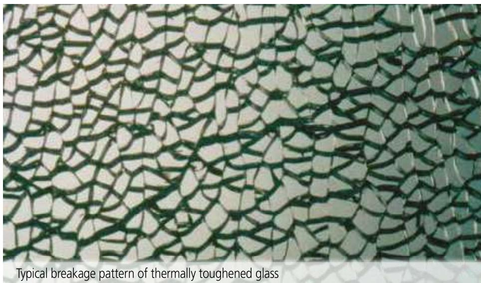
Typical breakage pattern of thermally toughened glass
