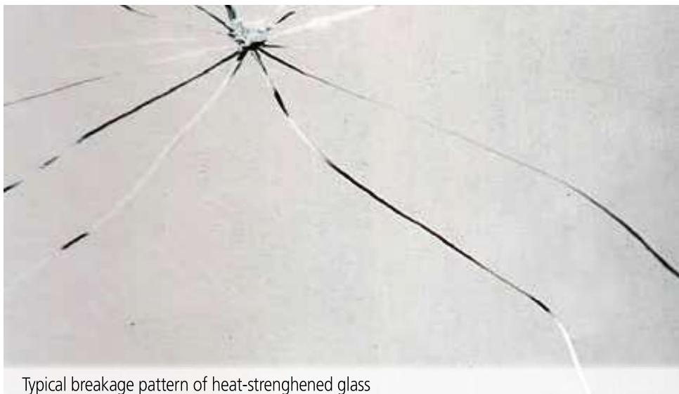
Typical breakage pattern of heat-strengthened glass
