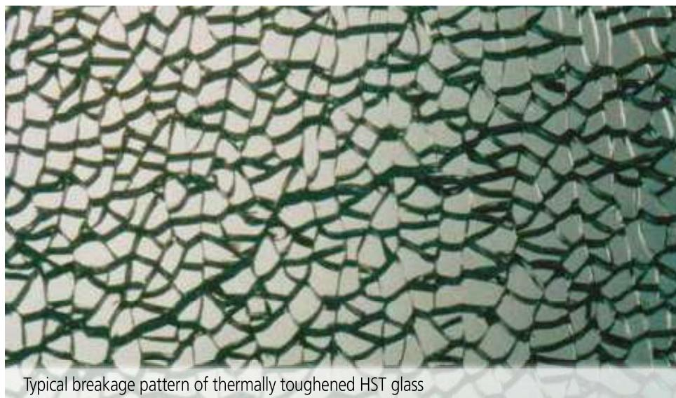
Typical breakage pattern of thermally toughened HST glass
